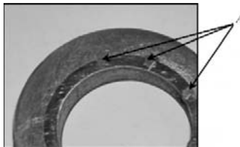
Figure 4. Macrosection of welded joint: A — places of the holes filled with aluminum
