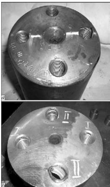
Figure 7. General view of the openings in new (base) (a) and repaired (b) journals of axle after the tests
