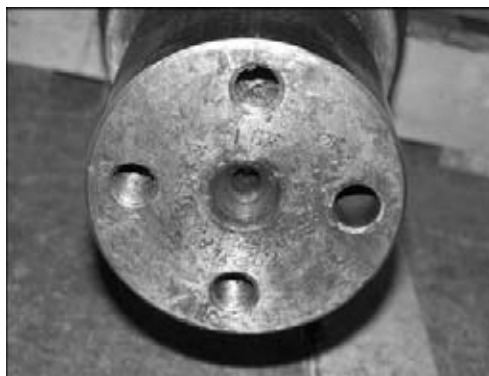
Figure 9. Repaired channel for thread cutting
