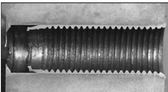
Figure 5. Macrosection of repaired threaded opening
