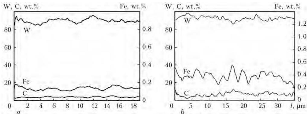
**Figure 1.** Curves of distribution of elements in non-spherical (a) and spherical (b) particles: *l* – length of a secant
