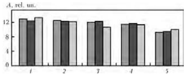
**Figure 2.** Diagram of wear resistance ( $A$ ) of samples clad with composite alloys with different contents of non-spherical tungsten carbide particles: 1 – 100 % of spherical particles; 2 – 80 % of spherical particles + 20 % of non-spherical particles; 3 – 50 % of spherical particles + 50 % of non-spherical particles; 4 – 100 % of non-spherical particles; 5 – 100 % of crushed tungsten carbide particles; 1–4 – powders produced by thermal centrifugal spraying
