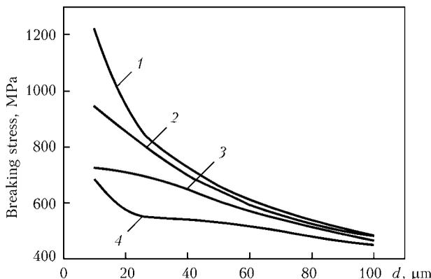
Figure 3. Dependence of breaking stress of grain of iron with bcc lattice on its size  $d$  at different temperatures: 1 – grain of metal without hydrogen at  $T = 350\text{--}250$ ; 2 – 350; 3 – 300; 4 – 250 K
