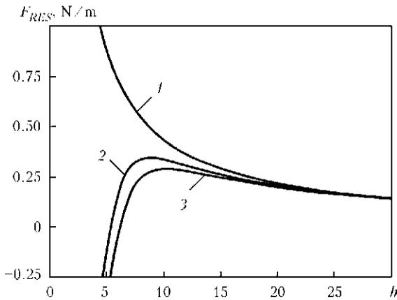
**Figure 1.** Dependence of resulting force of interaction of two edge dislocations  $F_{RES}$  on distance between them  $h$  (in modules of Burgers vector) at different concentration of diffusible hydrogen (metal temperature  $T = 300$  K) [17]: 1 – 0; 2 – 5; 3 – 10  $\text{cm}^3/100$  g
