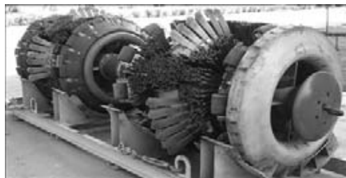
Figure 5. Magnetic in-pipe two-section flaw detector for transverse magnetisation with by-pass device
