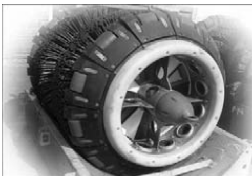
Figure 2. Cleaning magnetic in-pipe one-section piston with by-pass device
