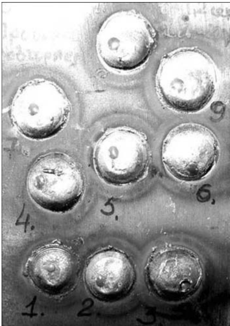
Figure 6. Appearance of spots produced by pulse electrode wire rate at 40 Hz frequency
