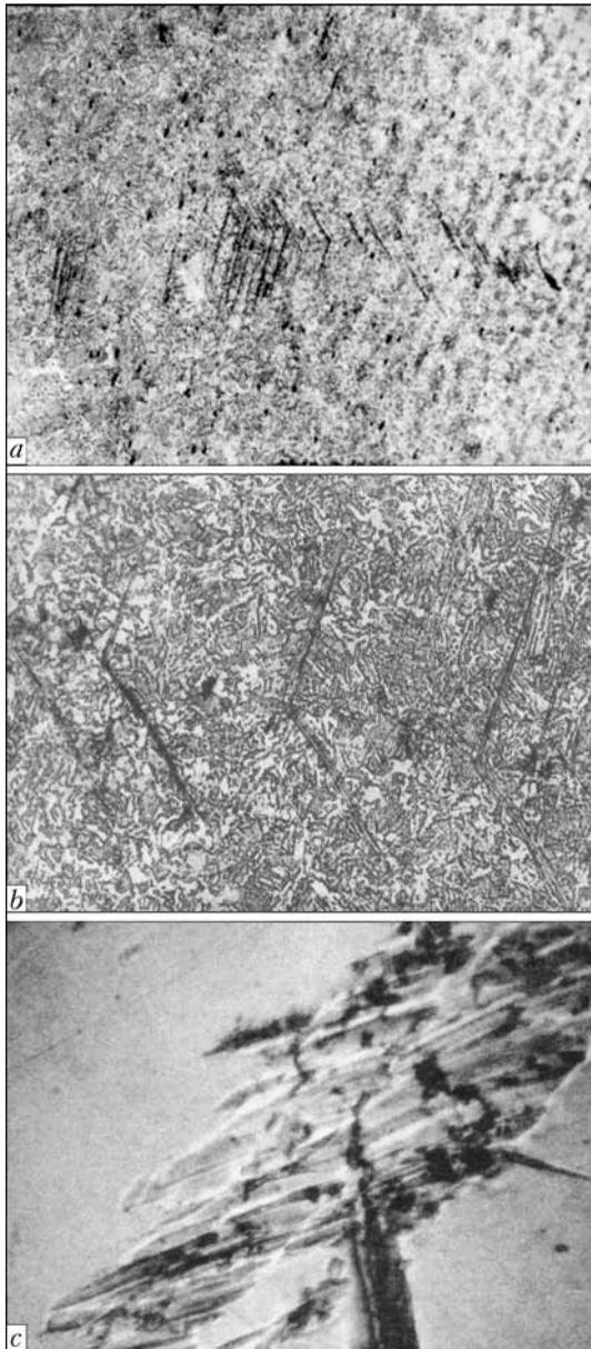
**Figure 2.** Slip bands, extrusions, intrusions in the metal of samples of 09G2S tee joints: *a, b* –  $N = 230,000$  cycles,  $\sigma_a = 120$  MPa; *c* –  $N = 720,000$  cycles,  $\sigma_a = 80$  MPa (*a* –  $\times 100$ ; *b* –  $\times 500$ ; *c* –  $\times 1000$ )
