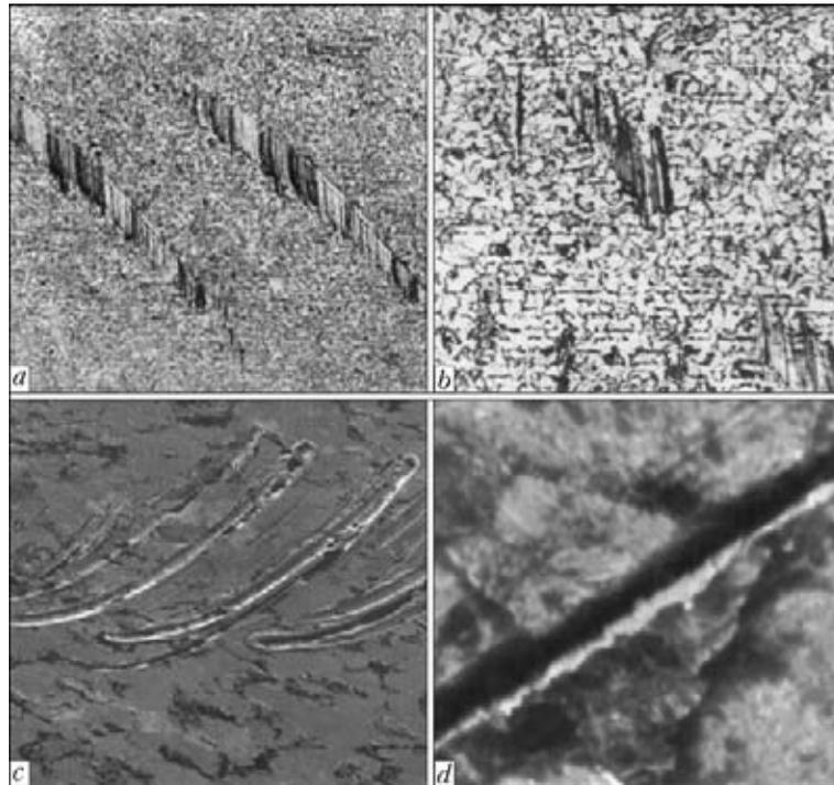
**Figure 6.** Microstructures with transverse microshears in samples of tee joints of 09G2S steel: *a* –  $\sigma_a = 120$  MPa,  $N = 400,000$  cycles; *b-d* –  $\sigma_a = 80$  MPa,  $N = 720,000$  cycles (*a* –  $\times 50$ ; *b* –  $\times 125$ ; *c* –  $\times 810$ ; *d* –  $\times 5000$ )
