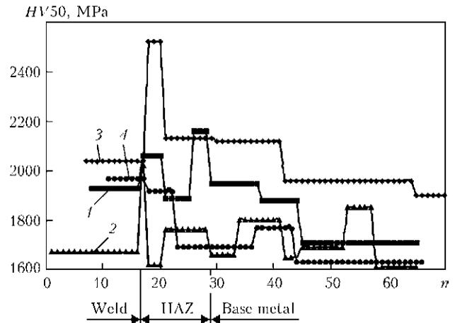
**Figure 5.** Microhardness of samples of tee welded joints of 09G2S steel after welding (1) and cyclic loading  $\sigma_a = 80$  MPa up to  $N = 400,000$  (2),  $700,000$  (3) and  $100,000$  (4) cycles:  $n$  – number of measurements
