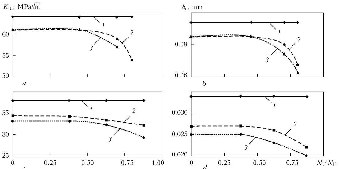
**Figure 1.** Change of  $K_{IC}$  (*a, c*) and  $\delta_c$  (*b, d*) values of HAZ metal of butt (*a, b*) and tee (*c, d*) welded joints of 09G2S steel with increase of the number of deformation cycles (cycle stresses for butt joints were 100 (*a*), 130 (*b*) MPa, and for tee joints – 80 (*c*), 120 (*d*) MPa): 1 –  $T_{test} = +20$  and  $-20$  °C; 2, 3 –  $T_{test} = -40$  °C
