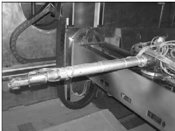
Figure 1. 90° turning system for repair and finishing smoothing of weld reverse bead
