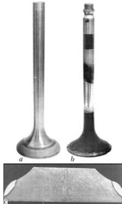
Figure 7. Surface appearance of 5D70 diesel engine valve, deposited using plasma-powder method with 50NKh25S5R alloy, immediately after surfacing ( a ) and after 5000 h of operation ( b ), and macrosection of deposited valve ( c )
