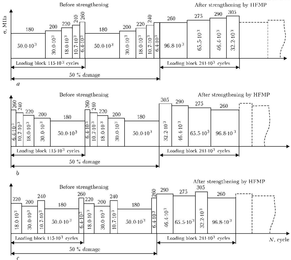
**Figure 3.** Diagram of loading of the T-joint specimens of steel 09G2S before and after strengthening in block loading with increasing (a), decreasing (b) and quasi-random (c) sequences of application of load in each block
