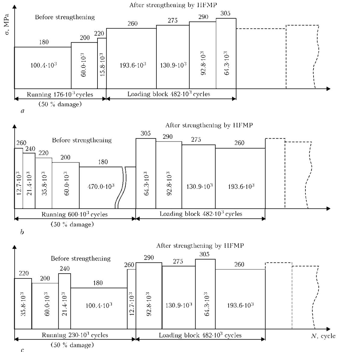
**Figure 2.** Diagram of loading of the T-joint specimens of steel 09G2S before and after strengthening under multistage loading with increasing (a), decreasing (b) and quasi-random (c) sequences of application of load
