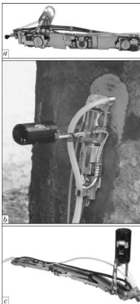
Figure 6. Appearance of robot with electromagneto-acoustic sensor (a), tool for abrasive cleaning (b) and welding torch (c)
