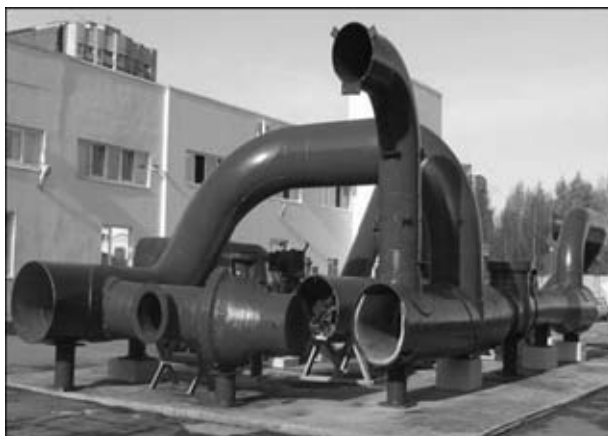
Figure 2. Test stand with artificial and natural defects
