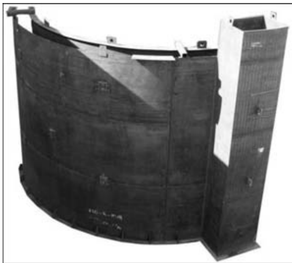
Figure 5. Test stand from steel S 223 of 20 mm thickness
