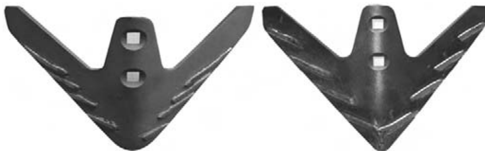
Figure 5. General view of hoe after local strengthening [10]
