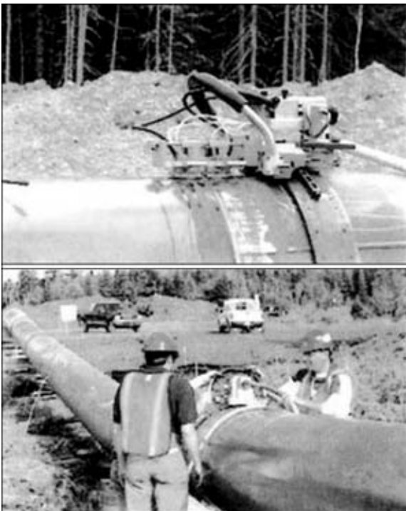
Figure 4. Pipe WIZARD-PA scanner
