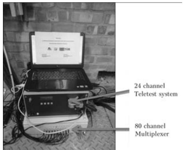
Figure 2. Tank floor structural health monitoring system
