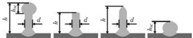
**Figure 5.** Different geometries of pins with characteristic dimensions
