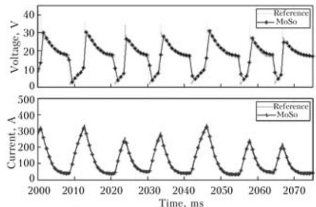
**Figure 3.** Current and voltage signal obtained by using MoSo and reference system: 19.0 V; 4 m/min, Ar + 25 % CO<sub>2</sub> and 1.0 mm ER70S-6 electrode
