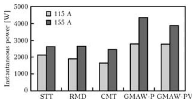
Figure 2. Instantaneous electric power for different GMAW processes
