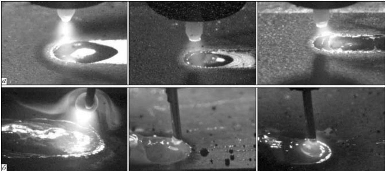
**Figure 4.** ViaSolda system images from left to right: *a* – GTAW at 250, 150 A (shorter exposure) and 150 A (longer exposure); *b* – GMAW at 150 A for globular transfer (30 V), short-circuit transfer during short-circuit (18 V) and short-circuit transfer during open arc (18 V)
