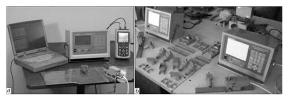
Figure 1. Ultrasonic computerized complex for residual and applied stress measurement: a — UltraMARS® model shown with a laptop and an oscilloscope; b — next generation UltraMARS®-7 model shown with all transducers, transducer holders and attachments
