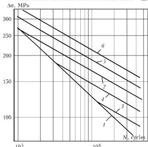
**Figure 4.** Fatigue curves of transverse loaded butt weld at R=0: line t-1 with high tensile residual stresses; lines t-1 with residual stresses equals to 0, 200, 100, -100 and -200 MPa, respectively
