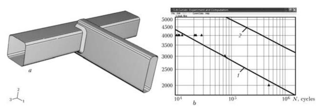
Figure 7. Fatigue curves (tendency) for tubular welded joints (as shown in the insert) showing the beneficial effect of UIT/UP: 1 — as-welded condition; 2 — after UIT/UP
