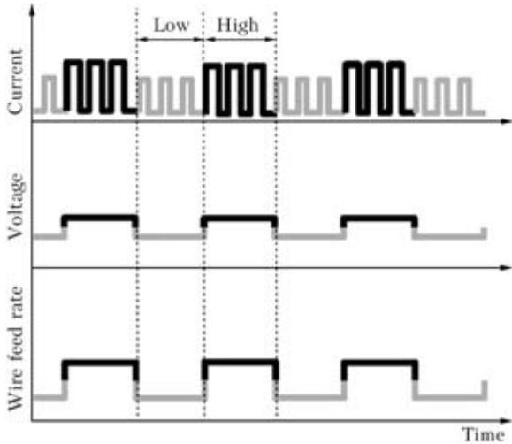
Figure 5. Low-frequency modulated pulsed GMA process
