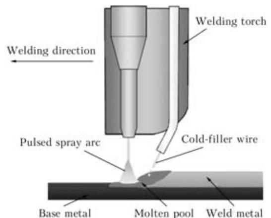
Figure 9. Principle of cold tandem pulsed GMA process
