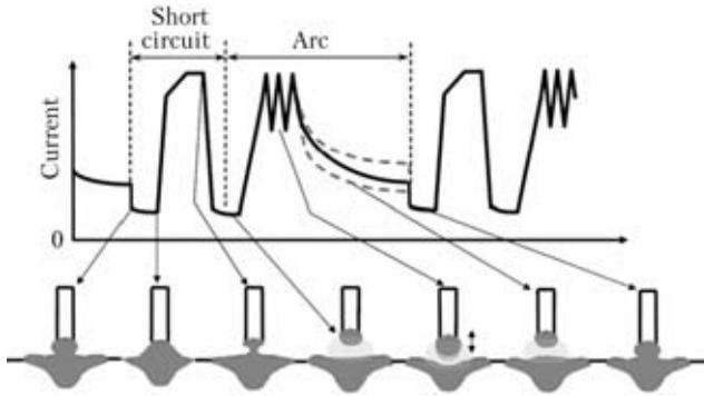
Figure 3. Controlled bridge transfer expanded (CBT expanded) process
