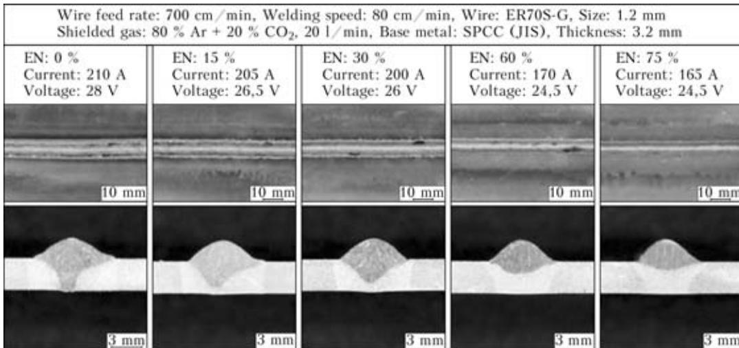
Figure 8. Effect of EN ratio on bead formation
