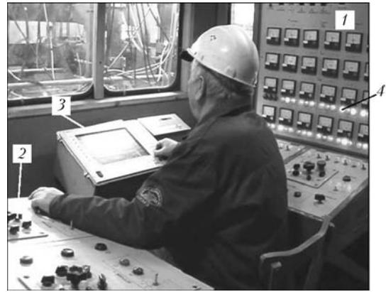
**Figure 3.** Central cabin of control of installation machines: 1, 2 – respectively, control panels of right and left blocks; 3 – industrial computer PC 670 of system of welding conditions monitoring; 4 – signal lamps of control of welding wires movement
