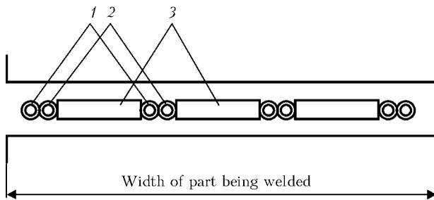
**Figure 2.** Scheme of consumable nozzles with channels for wire feeding (variant for one phase): 1, 2 – channels for movement of working and doubling welding wires, respectively; 3 – plates of consumable nozzle
