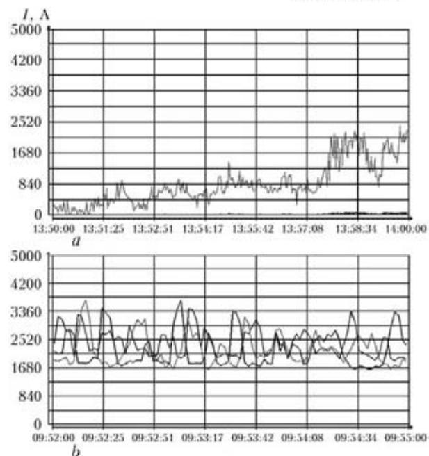
**Figure 6.** Oscillograms of welding current for single-phase of consumable nozzle at the area of weld after 50 min since the welding beginning ( $v_{w.f} = 115$  m/h) (*a*) and three-phase scheme of consumable nozzles after 32 min since the welding beginning ( $v_{w.f} = 150$  m/h) (*b*)
