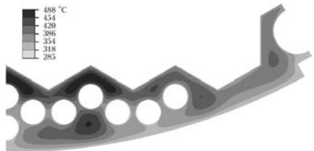
Figure 7. Temperature distribution in reactor reflection shield at operation at maximum power
