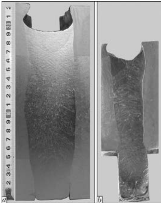
Figure 5. Macrostructures of welded joints (longitudinal section) produced using standard (a) and narrow-gap ESW (b)
