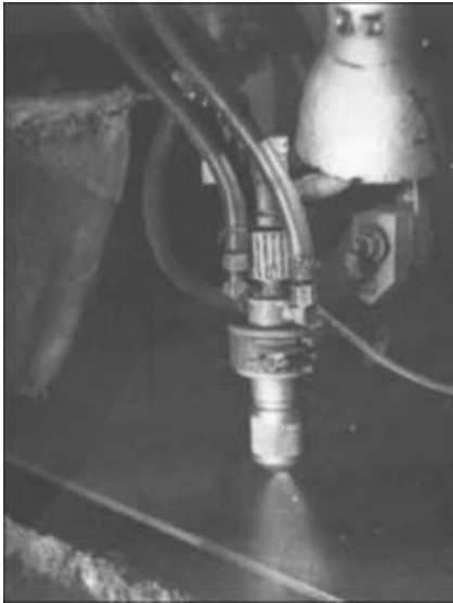
Figure 3. Plasmatron PMR 74M for cutting (plasma-forming medium – air + water)
