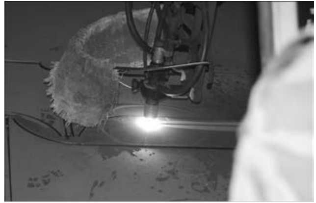
Figure 4. Process of cutting (plasma-forming medium – air + water)
