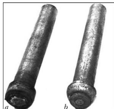
**Figure 5.** Billets of rods of DN 50 valves surfaced by manual arc (a) and plasma (b) processes
