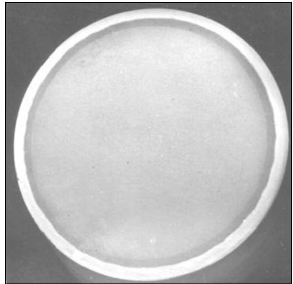
**Figure 4.** Transverse macrosection of cylindrical part of the rod of DN 50 gate valve surfaced by plasma-powder process
