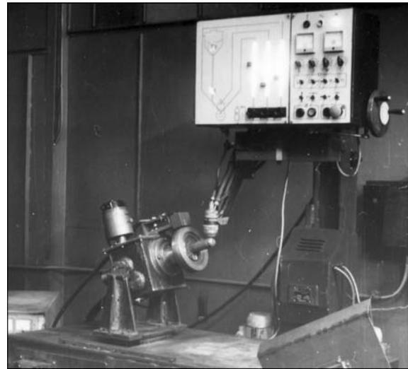
Figure 6. Unit for treatment of sealing surfaces of valve rods
