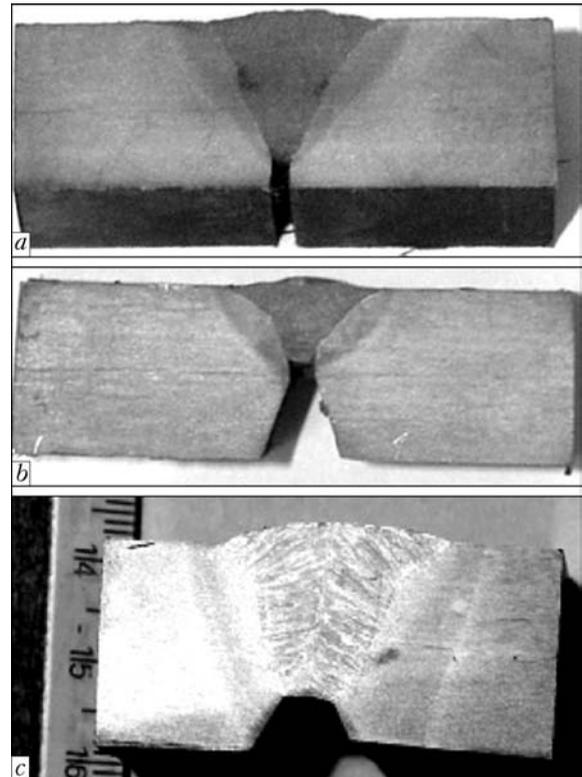
**Figure 8.** Typical macrosections manufactured of technological samples «rigid contour welding» of steel 06GBD: *a, b* – mechanized welding in shielding gases; respectively, V- and X-shaped preparation of edges 12 mm thick; *c* – automatic submerged arc welding; X-shaped preparation of edges 20 mm thick
