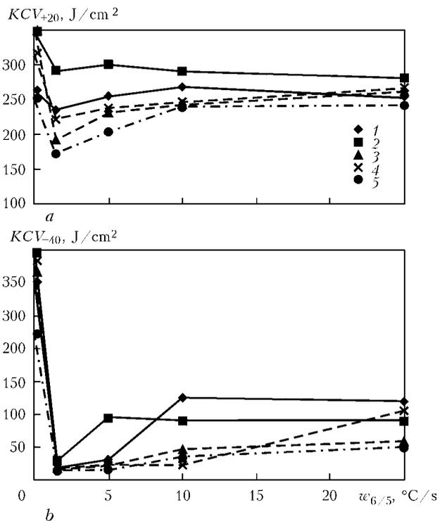
**Figure 5.** Dependence of impact toughness KCV for  $T_{test} = +20$  (a) and  $-40$  (b) °C of steel 06GBD HAZ metal on cooling rate at different thickness of rolled metal  $\delta = 12$  (1), 14 (2), 20 (3), 32 (4) and 40 (5) mm
