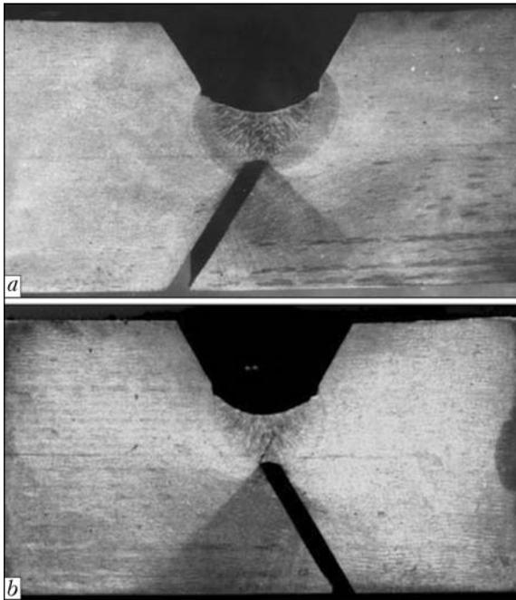
**Figure 6.** Sections of Tekken samples produced using electrodes UONI-13/55 at  $[H]_{diff} = 10$  (a) and 15 (b) ml/100 g
