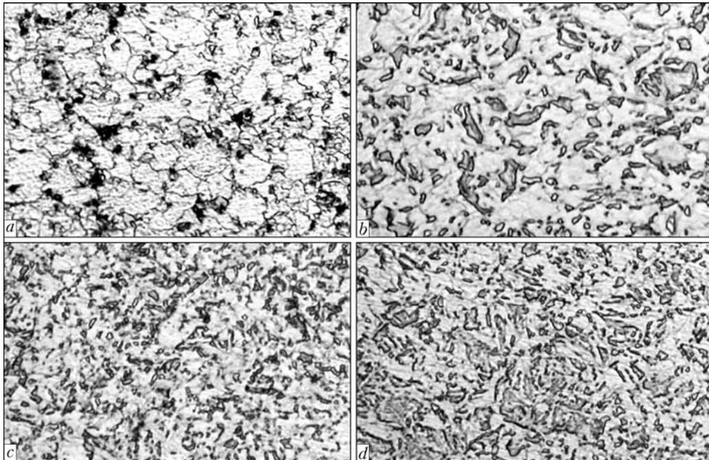
**Figure 2.** Microstructures ( $\times 500$ ) of steel 06GBD specimens at  $w_{6/5} = 1.3$  (a), 10.1 (b), 27 (c) and 70 (d)  $^{\circ}\text{C}/\text{s}$
