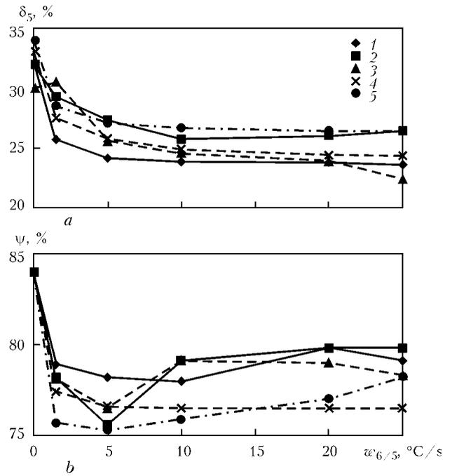
**Figure 4.** Dependence of relative values of elongation (a) and reduction in area (b) of HAZ metal of steel 06GBD on cooling rate of metal of different thickness  $\delta = 12$  (1), 14 (2), 20 (3), 32 (4) and 40 (5) mm
