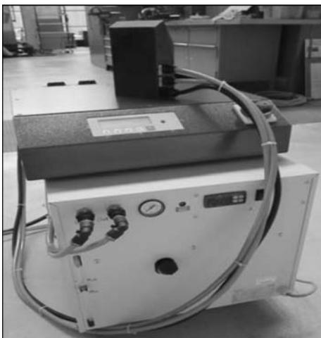
**Figure 5.** Coaxial coil KI-112-U-30° with pulse generator EW100W and chiller
