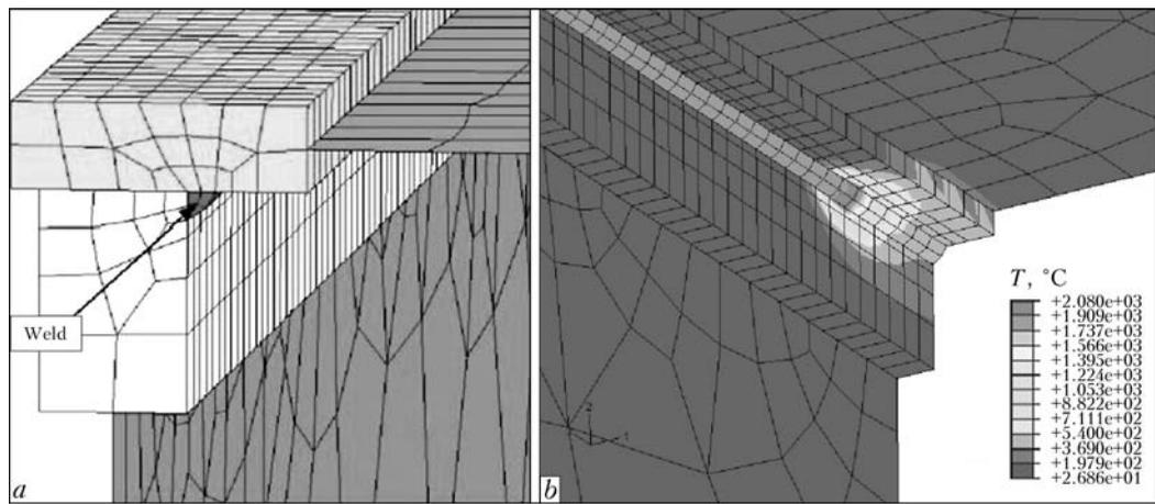
Figure 6. Software «Abaqus»: a – finite element model of weldment; b – distribution of thermal fields
