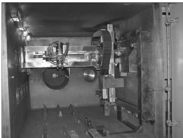
Figure 2. Unit of modified welding EB gun with the mechanisms of movement along coordinates X , Y , Z and inclination on the coordinate VG
