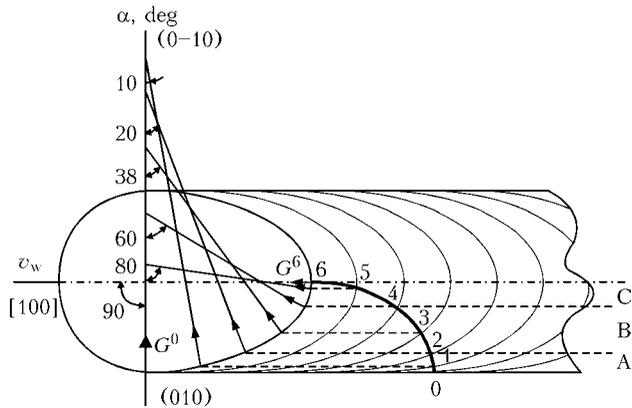
**Figure 2.** Schematic image of the change of direction of maximum temperature gradient  $G$  over weld pool solidification front: A, B, C – characteristic structural zones of the weld;  $\alpha$  – deviation angle  $G$
