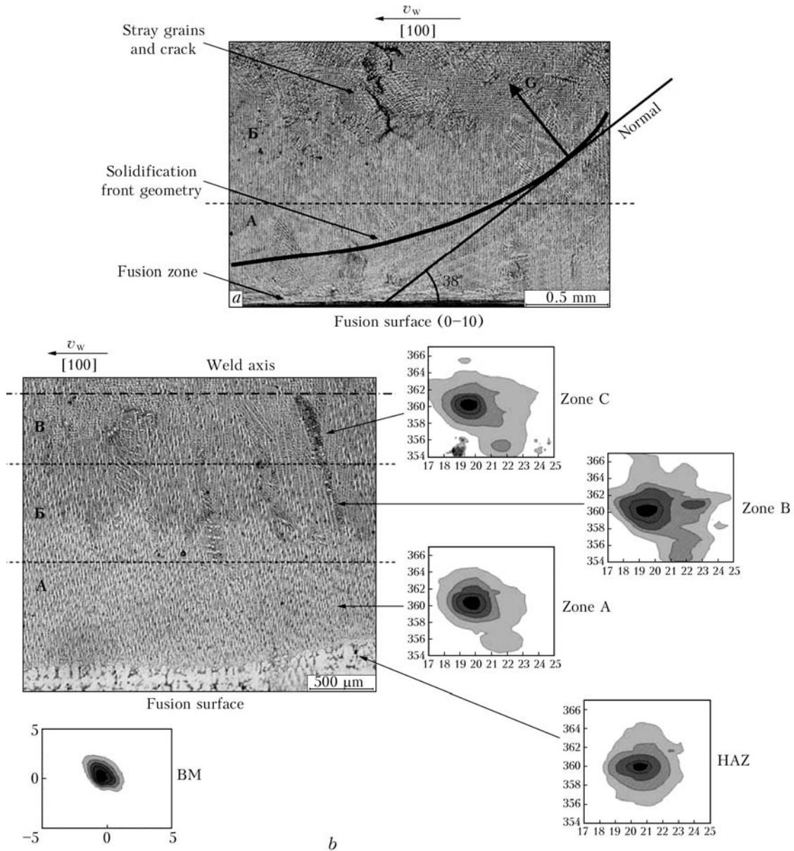
**Figure 3.** Microstructure (a) and isointensive  $I_{q\perp}$  curves (b) of weld metal zones corresponding to different deviations from maximum temperature gradient over weld pool solidification front (acc. to Figure 2) (numerical values along zone axes are shown in degrees)
