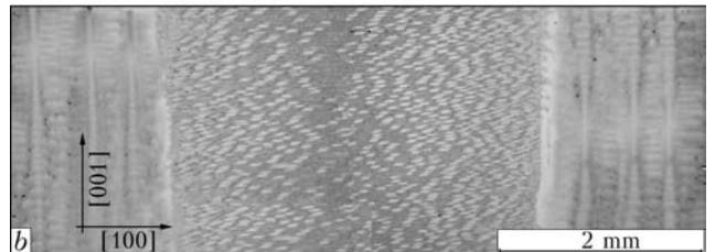
**Figure 7.** Appearance (a) and microstructure of single-crystal weld (b) of JS32 alloy made with control of weld pool solidification:  $\alpha$  – angle of deviation of weld pool solidification macrofront from {100}
