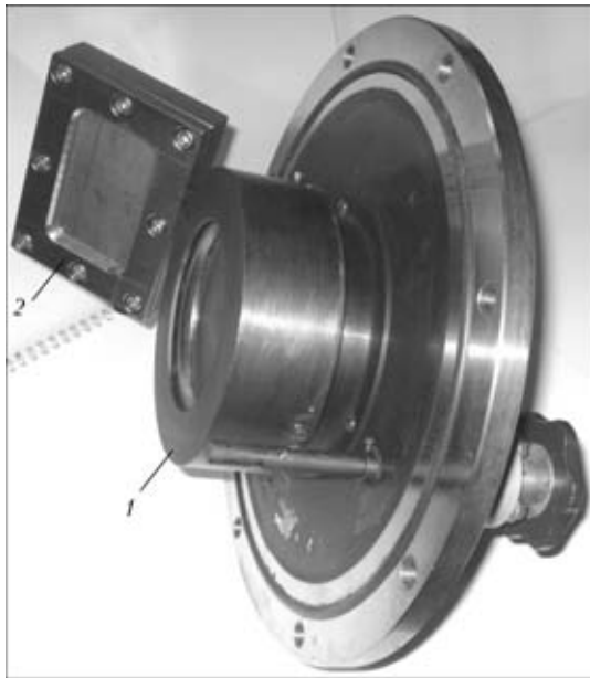
Figure 2. Module of magnetron sputtering, consisting of Magnetron 1 (1) and Magnetron 2 (2)
