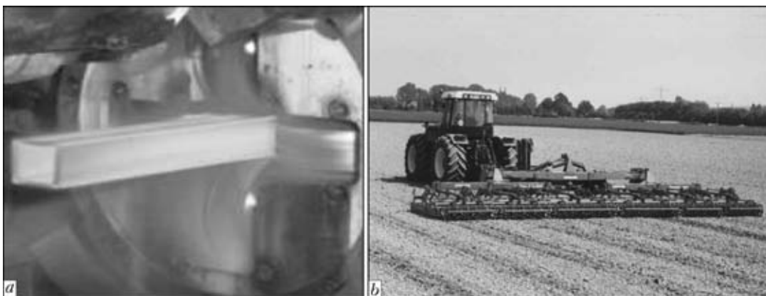
Figure 1. Production of square MSH-sections in the last rolling stand (a), and their application in agricultural machinery engineering (b)
