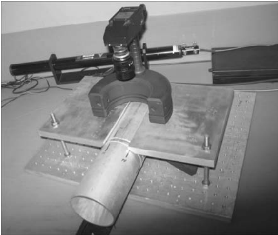
Figure 3. Device and specialized fixture for measurement of residual stresses of welded circumferential joints of AMg6 alloy using method of speckle-interferometry
