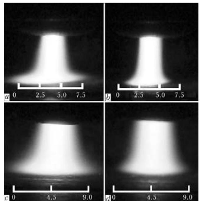
**Figure 6.** Appearance of a microplasma arc with effective thermal power of 341 W at different degrees of arc constriction by microplasmatron nozzles: *a* –  $d_{pl} = 1.8$  mm,  $d_f = 2.5$  mm, shielding gas – Ar; *b* –  $d_{pl} = 1.8$  mm;  $d_f = 2.5$  mm, shielding gas – 90 % Ar + 10 % H<sub>2</sub>; *c* –  $d_{pl} = 2.5$  mm,  $d_f = 4.5$  mm, shielding gas – Ar; *d* –  $d_{pl} = 2.5$  mm;  $d_f = 4.5$  mm, shielding gas – 90 % Ar + 10 % H<sub>2</sub>. Distance to anode is 5 mm
