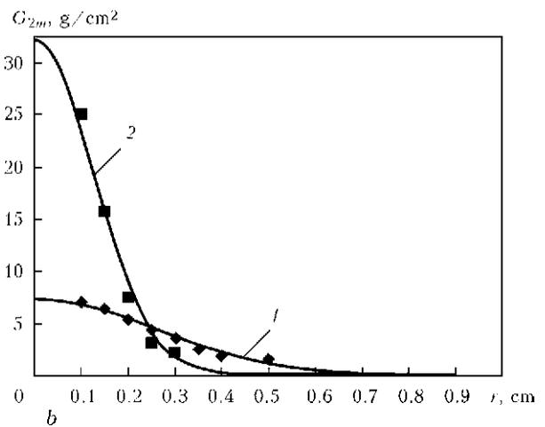
**Figure 3.** Schematic of two-phase microplasma-filler powder flow over two-section powder catcher (a) and calculated distribution of fed powder by a normal law in anode plane (b): 1 –  $d_{pl} = 2.5$  mm,  $d_f = 4.5$  mm; 2 –  $d_{pl} = 1.8$  mm,  $d_f = 2.5$  mm; symbols – experimental data, solid curve – simulation
