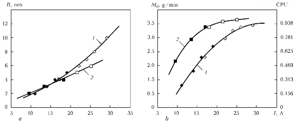
**Figure 1.** Dependence of bead width  $B$  (a), deposited metal specific mass  $M_d$  and CPU (b) on welding current  $I$  at  $v_d = 2.75$  m/h (flow rate of carrier gas (argon) 2.5; shielding gas (mixture of 90 % Ar + 10 % H<sub>2</sub>) 7 l/min; base metal – austenitic stainless steel); 1 – microplasmatron with  $d_{pl} = 2.5$  mm,  $d_f = 4.5$  mm; 2 –  $d_{pl} = 1.8$  mm;  $d_f = 2.5$  mm; dark symbols – deposition on a narrow substrate; light ones – deposition on a wide substrate
