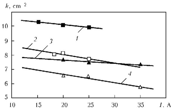
**Figure 5.** Dependence of coefficient of concentration of specific heat flow  $k$  into microplasma arc anode on welding current: 1 –  $d_{pl} = 1.8$  mm;  $d_f = 2.5$  mm, shielding gas – 90 % Ar + 10 % H<sub>2</sub>; 2 –  $d_{pl} = 1.8$  mm;  $d_f = 2.5$  mm, shielding gas – Ar; 3 –  $d_{pl} = 2.5$  mm;  $d_f = 4.5$  mm, shielding gas – 90 % Ar + 10 % H<sub>2</sub>; 4 –  $d_{pl} = 2.5$  mm;  $d_f = 4.5$  mm, shielding gas – Ar
