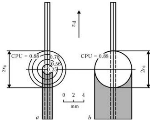
**Figure 4.** Features of cladding of a narrow substrate 1 mm wide at application of microplasmatron with  $d_f = 4.5$  mm with insufficient concentration of two-phase microplasma-filler powder flow: *a, b* – see the text
