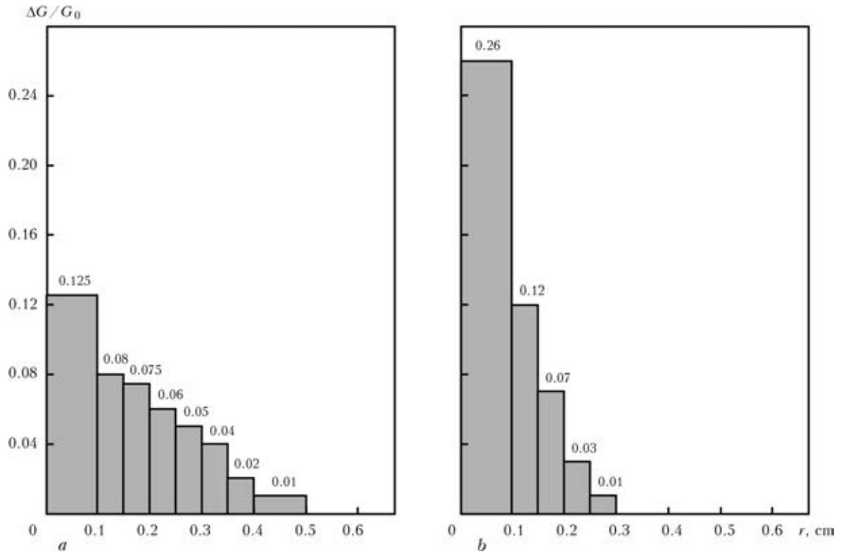
**Figure 2.** Histogram of fed powder distribution in the direction normal to deposited bead axis, depending on parameters of PPS-004 microplasmatron: *a* –  $d_{pl} = 2.5$  mm,  $d_f = 4.5$  mm; *b* –  $d_{pl} = 1.8$  mm;  $d_f = 2.5$  mm
