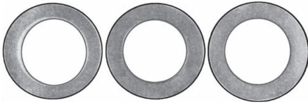
**Figure 3.** Cross-section of MTT strengthened LRS tubes after 21 thou h of operation
