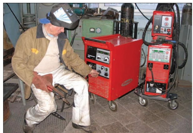
Figure 2. Application of inverter arc power sources with corresponding feeder for flux-cored wire welding
