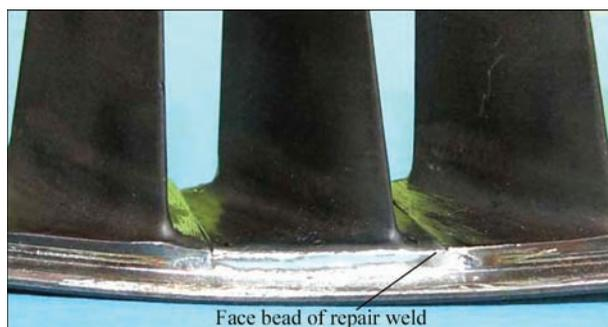
**Figure 13.** View of repair joint from end of guide case semi-ring nor-blade base. It is a result of difficulty of local mechanical removal of the damaged blade and formation of the area for the donor-blade. Such gaps are very critical, since thickness of the wall, to which the blade is welded, makes only 0.5 mm in some places.
