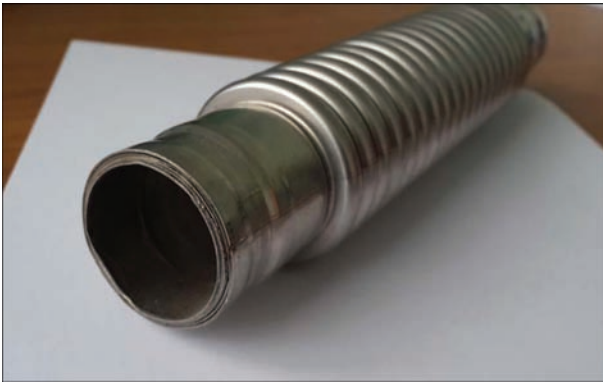
Figure 3. Appearance of billet of multilayer bellows after hydroforming
