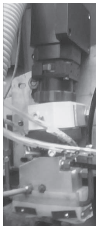
Figure 10. Appearance of developed working head for laser, microplasma and hybrid laser-microplasma welding
