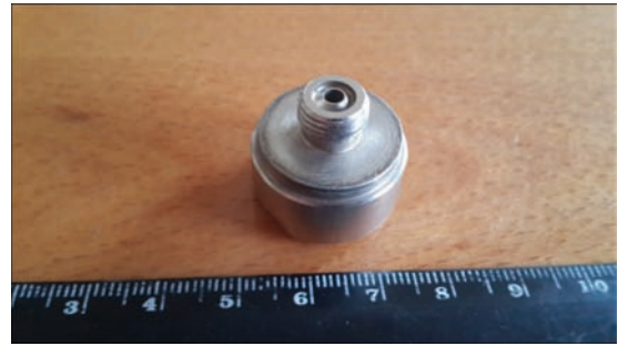
Figure 12. Housing of probe from steel 08Kh18N10T welded by laser radiation
