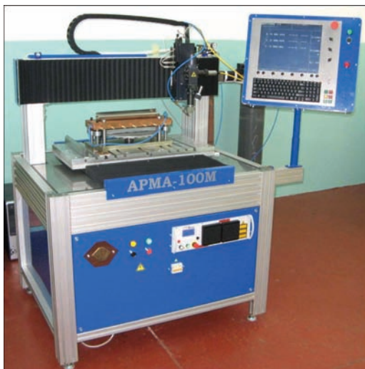
Figure 4. Appearance of three-coordinate complex «ARMA-100M» for laser welding
