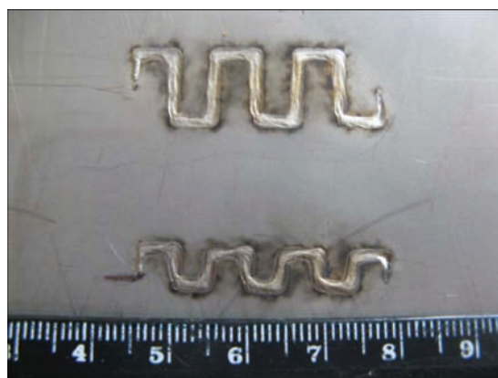
Figure 9. Appearance of welds produced on curved trajectory using instrument for manual laser welding
