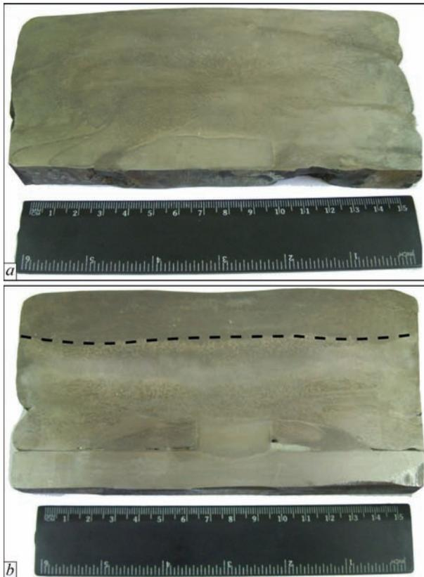
**Figure 5.** Longitudinal macrosection of a bimetal billet, produced by surfacing with 90 mm electrode at  $N_{\text{CSM}} = 80\text{--}90$  (a) and 130 kV·A (b) (dashed line marks the shape of metal pool in the deposited metal)
