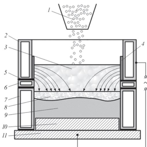
**Figure 2.** Shape of metal pool produced at ESS in CSM with discrete filler (arrows show current distribution in CSM): 1 — discrete filler; 2, 6, 7 — current-conducting, intermediate and forming sections of the mould, respectively; 3 — slag pool; 5 — insulating interlayer; 8 — metal pool; 9 — deposited metal; 10 — billet; 11 — tray
