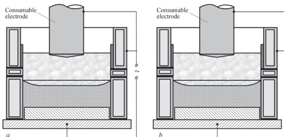
**Figure 3.** Electric circuits of remelting electrode connection at the same (a) and different from CSM (b) potential
