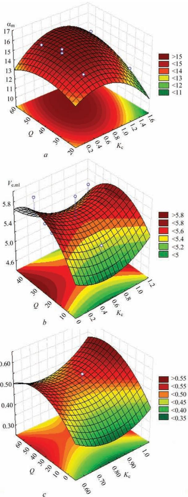
**Figure 3.** Dependence of melting coefficient  $\alpha_m$  (a), rate of electrode melting  $V_{e,m}$  (b) and electrode coating  $V_{coat}$  (c) on amount of exothermal mixture  $Q$  and coefficient of electrode coating mass  $K_c$  in electroslag remelting (ESR) or casting into crucible in electroslag die casting (EDC). However, laboriousness of ingot casting taking into account time of flux melting in flux-melting furnaces is significantly higher in comparison with «solid» start.
