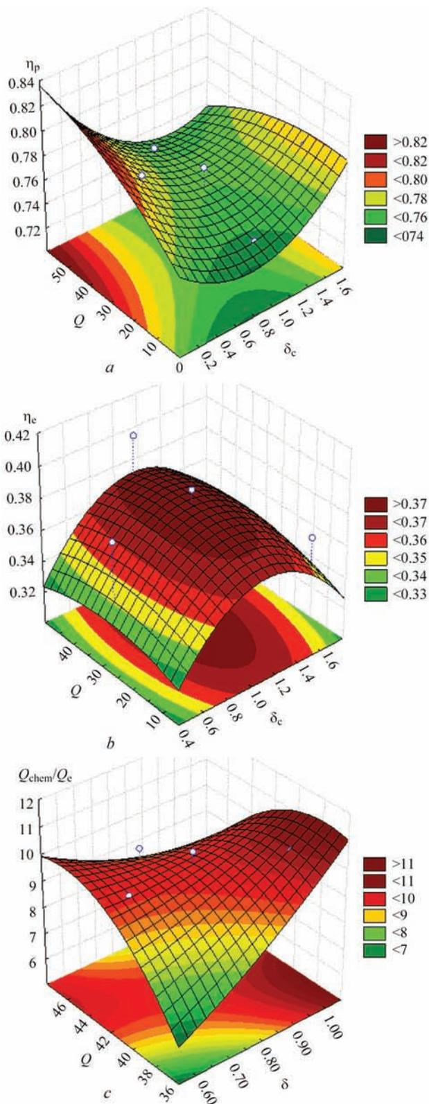
**Figure 4.** Dependence of heating efficiency of part  $\eta_p$  (a), electrode  $\eta_e$  (b) and relationship of heats  $Q_{chem}/Q_e$  (c) on amount of exothermal mixture  $Q$  and electrode coating thickness  $\delta_e$
