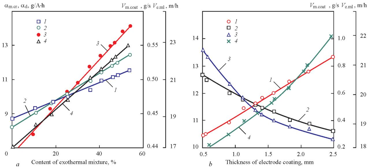
**Figure 1.** Variation of indices of electrode melting depending on amount of exothermal mixture (a) and coating thickness (b) in the coating
