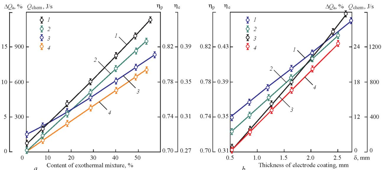
**Figure 2.** Effect of amount of exothermal mixture in the electrode coating (a) and coating thickness (b) on melting heat characteristics
