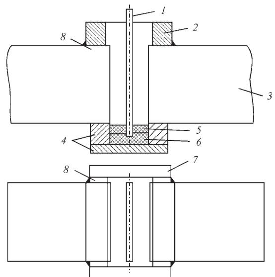
**Figure 5.** ESW scheme: 1 — plate electrode; 2 — run-off tabs; 3 — welded joint; 4 — metallic pocket; 5 — working flux; 6 — exothermal mixture; 7 — forming backgigs; 8 — side plates
