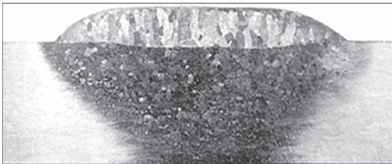
Figure 6. Macrosection of joint, deposited by a flux-cored wire PPT-22 on VT22 alloy plate in as-surfaced state
