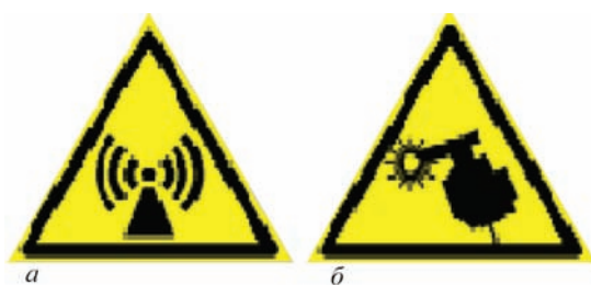
Figure 3. Hazard warning signs «Caution. Non-ionizing radiation» (a) and «Caution. Welding» (b)
