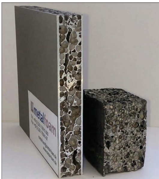
Figure 1. Porous aluminium panels produced by MetalFoam Company with and without monolithic walls
