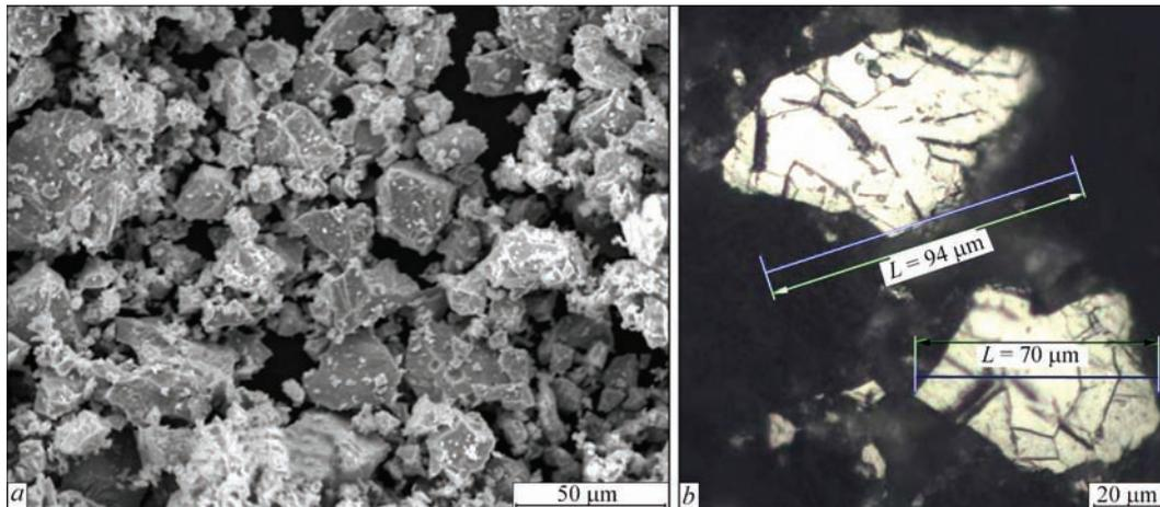
Figure 4. Appearance (a) and microstructure (b) of HDH powder VT1-0 of 63–100  $\mu\text{m}$  fraction, used for deposition
