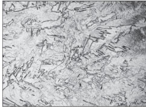
**Figure 10.** Microstructure ( $\times 100$ ) of metal of deposited outer layers
