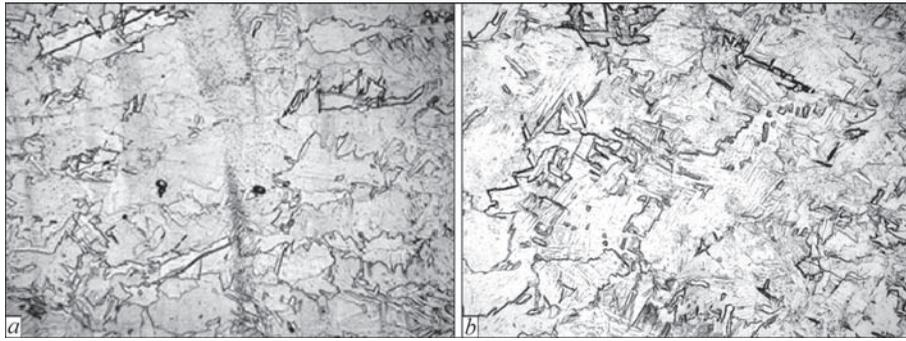
**Figure 11.** Microstructure of deposition in central part of specimen: *a* —  $\times 200$ ; *b* —  $\times 100$
