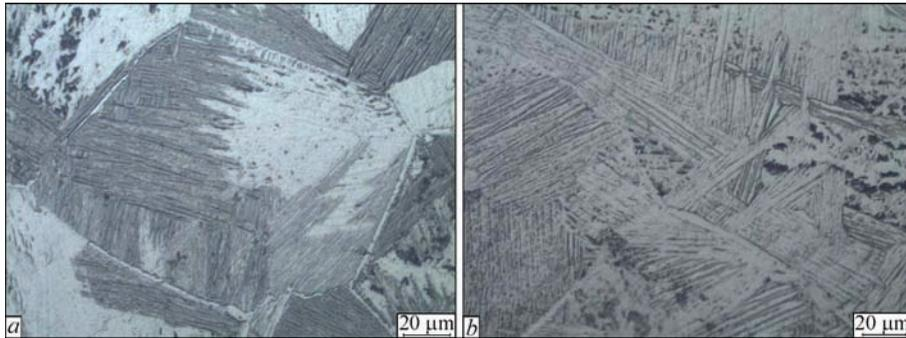
**Figure 12.** Microstructure of layers: *a* — layer 350; *b* — 120  $\mu\text{m}$
