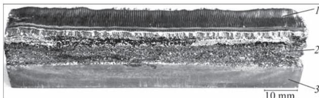
Figure 5. Specimen of part, made by electron beam 3D-deposition method: 1 — upper layer of deposited metal; 2 — interlayer of metal with particles of unmelted powder; 3 — titanium substrate
