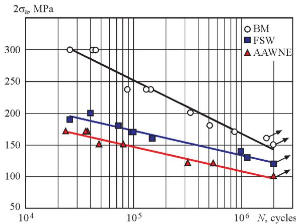
**Figure 6.** Curves of fatigue of base material and welded joints of aluminium alloy D16 of 2 mm thickness at the asymmetry of loading cycle  $R_{\sigma} = 0.1$  (BM — base metal)
