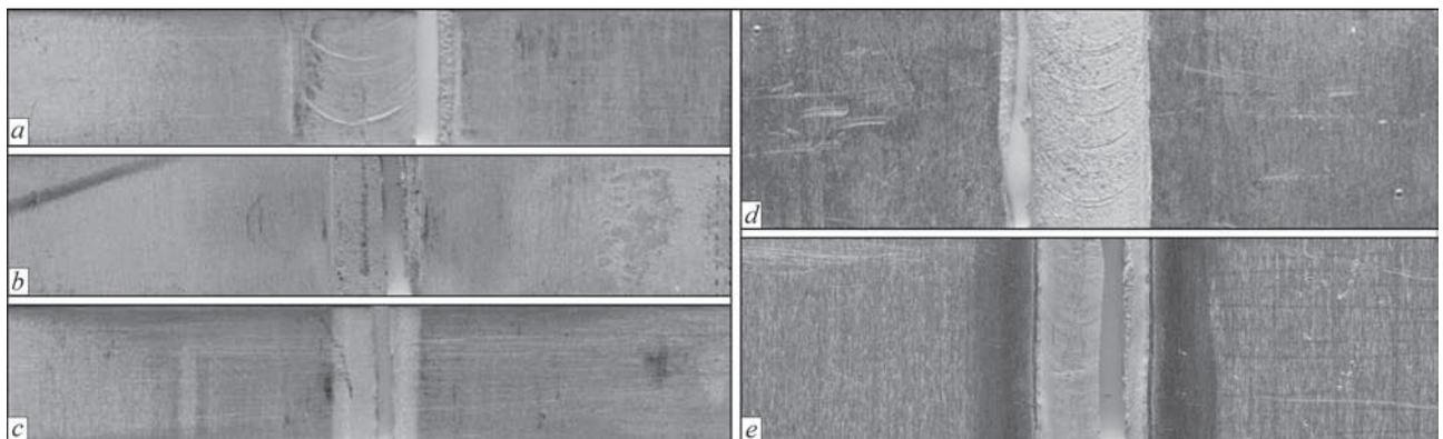
**Figure 5.** Fragments of specimens of welded joints produced using FSW (a, d) and AAWNE (b, e — with weld reinforcement; c — without weld reinforcement) fractured at uniaxial static tension (a–c) and cyclic load (d, e)
