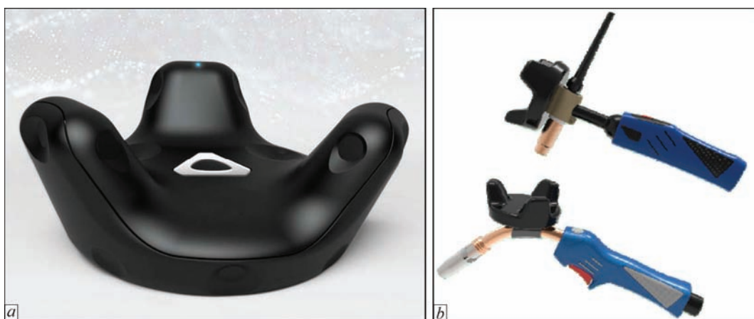
Figure 5. Application of Vive tracker controller for modeling virtual welding torches based on real ones and tracing their movement in space: a — Vive tracker controller; b — real welding torches with controllers put on them
