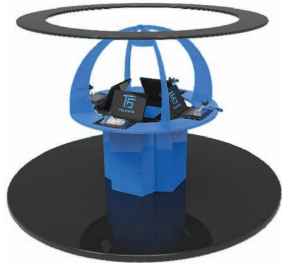
Figure 10. Design of virtual training station with four welding trainers V60
