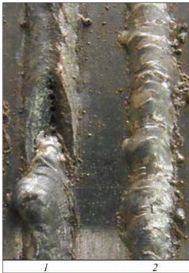
Figure 1. Appearance of deposited beads: 1 — regular wire feed; 2 — modulated feed
