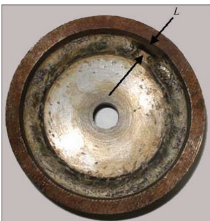
Figure 2. Appearance of pipe cap with welded-in plug: L — real gap between the cap and pipe
