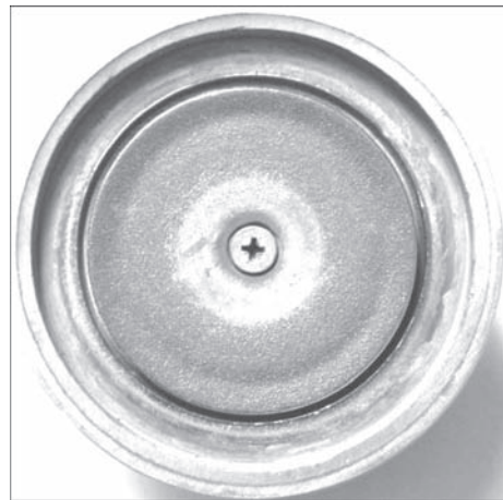
Figure 2. Compound target Al + Fe with insert ( d = 64 mm, \delta = 3 mm) of steel St.3
