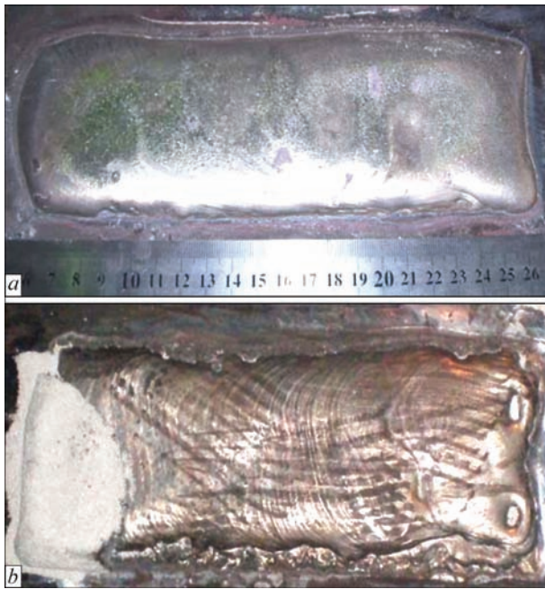
Figure 5. Influence of gap between the strips l on formation of deposited metal: a — l = 8 mm; b — 16 mm. Surfacing mode: I_s = 1200 – 1300 A; U_s = 32 – 33 V; v_s = 14 m/h
