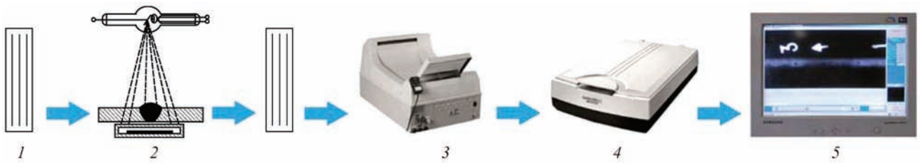
Figure 1. Traditional scheme of radiography testing using film and digitization of radiographs: cassette charging (1); exposure on X-ray film (2); procedure of film treatment (3); film scanning (4); DI (5)
