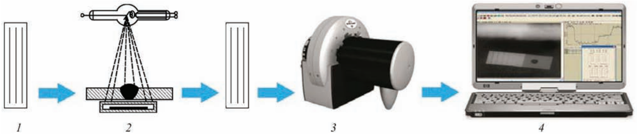
Figure 2. Scheme of exposure procedure using memory plate: preparation of cassette with memory plate (1); exposure on memory plate (2), reading from plate (3); DI (4)
