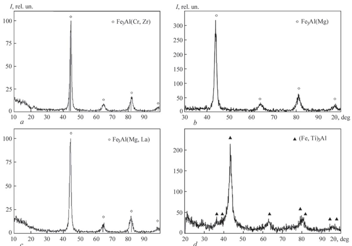
**Figure 7.** X-ray patterns of powders produced by MCS method in planetary mill during 5 h of mixtures (wt.%): *a* — 86 Fe + 14 Al1.5Cr1Zr; *b* — 86 Fe + 14 Al5Mg; *c* — 86 Fe + 14 Al5Mg1La, *d* — 60.8 Fe + 39.2 TiAl
