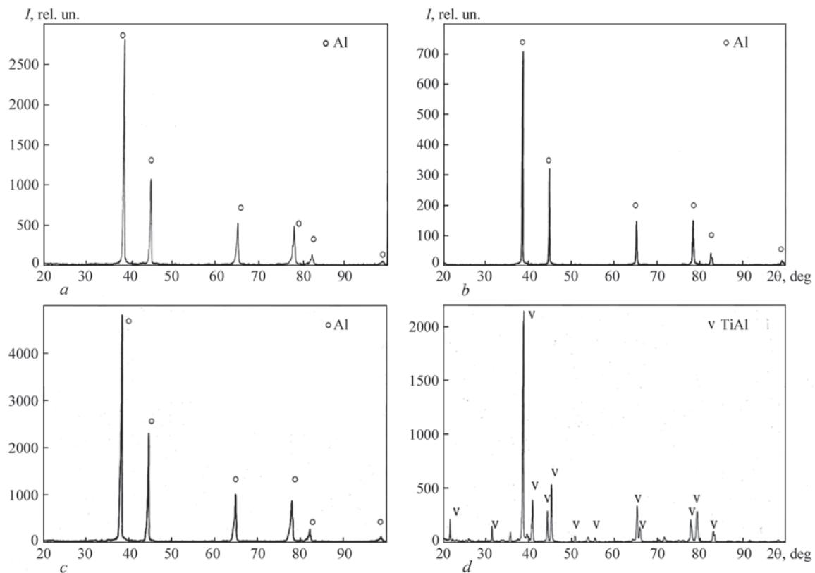
**Figure 2.** X-ray patterns of powders of aluminum alloys: *a* — Al<sub>1.5</sub>Cr<sub>1</sub>Zr; *b* — Al<sub>5</sub>Mg; *c* — Al<sub>5</sub>Mg<sub>1</sub>La; *d* — Ti<sub>35</sub>Al
