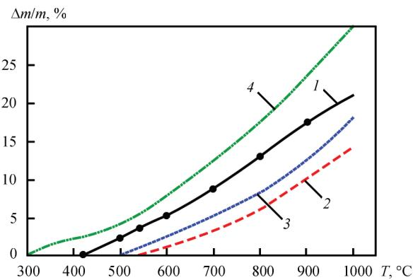
**Figure 10.** Specific increase of weight of powders in heating on air: 1 —  $\text{Fe}_3\text{Al}$ ; 2 —  $\text{Fe}_3\text{Al}(\text{Cr}, \text{Zr})$ ; 3 —  $\text{Fe}_3\text{Al}(\text{Mg})$ ; 4 —  $(\text{Fe}, \text{Ti})_3\text{Al}$
