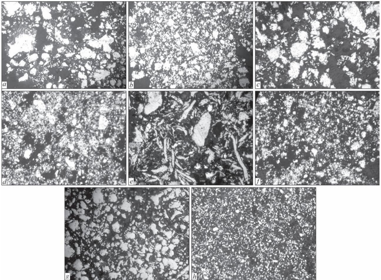
**Figure 3.** Microstructure ( $\times 400$ ) of particles of alloyed powders produced from charge: 86 Fe+14 Al1.5Cr1Zr (*a, b*), 86 Fe + 14 Al5Mg (*c, d*), 86 Fe + 14 Al5Mg1La (*e, f*), 60.8 Fe + 39.2 TiAl (*g, h*), in planetary mill during 0.5 (*a, c, e, g*) and 5.0 h (*b, d, f, h*)
