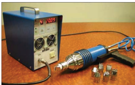
Figure 5. System for ultrasonic peening, increasing the fatigue life of welded elements and structures [8]
